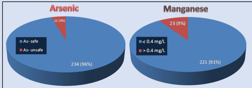
**Figure 8. Success rate of the 245 wells installed in the intermediate deep aquifers (IDTW) in Matlab, Bangladesh.**
