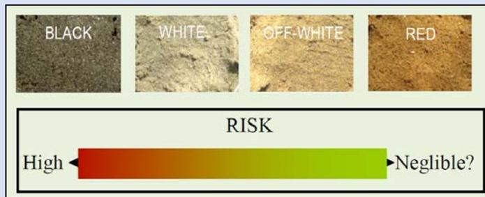
**Figure 5. Local drillers' perception of sediment colour and identification of safe aquifers for well installations.**
