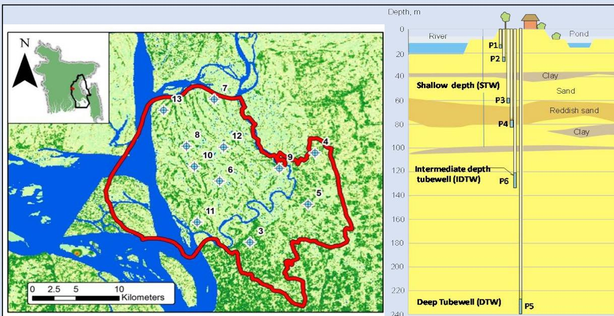
**Figure 7. Schematic sketch for assessment of hydrogeological suitability for installation of piezometer nests (groundwater observation well-nests) at shallow, intermediate and deep aquifers in Matlab, Bangladesh.**
