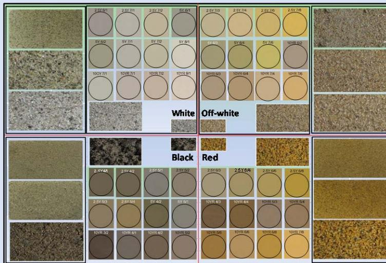
**Figure 6. A prototype of the simplified colour tool for the use of local drillers for targeting safe aquifers at shallow depths (< 100m).**
